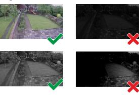
Any shadow cones or frequent changes of lighting could cause problems in detection.
